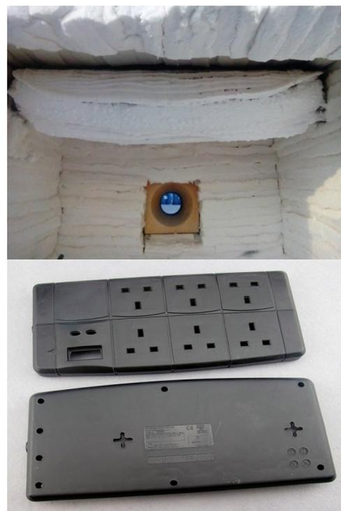
*Photos: Top: furnace test of cellulose insulation material with Presafar PIN FR. Below: Application of Presafar PIN FR in an electrical socket unit.*
