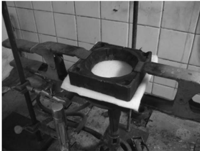
**Figure 4** Meeker burner test set-up for studying char characteristics.
